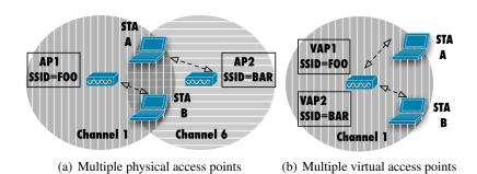
Figure 1: Virtualizing Access Point
