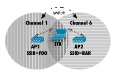
Figure 2: Multiple virtual STAs (with channel switu
