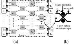
Figure 2:  $NXN\lambda$ -router architecture (a), 4-port optical switch architecture example (b).
