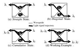
Figure 3: Functional States of a 4-port Optical Switch
