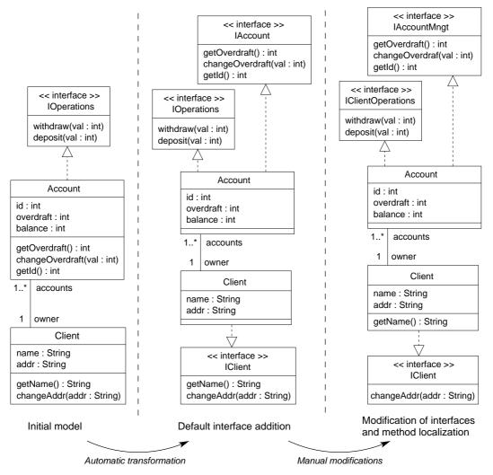
Figure 2: Refinement example: addition and modification of interfaces
