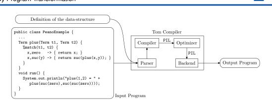
Figure 1: General architecture of Tom: the compiler generates an intermediate PIL program which is optimized before being pretty-printed by the back-end into the host-language.
