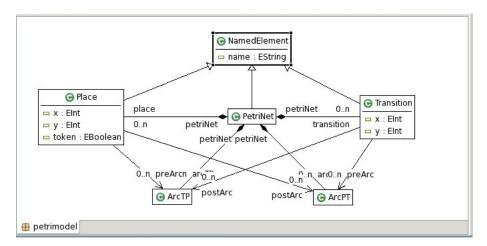
Figure 2: Petri net model after refactoring
