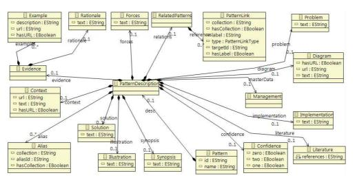
Figure 2: Overview of the meta-model of PLML
