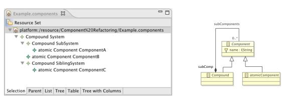
Figure 1: Example of Hierarchical Component Model and Corresponding Conceptual Model
