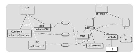
Figure 7: Model-to-text transformation after application of rule transformCALLS
