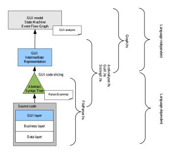
Figure 1: GUISurfer Architecture and Retargetability
