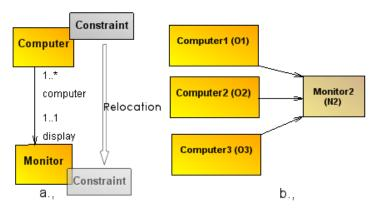
Figure 5: *MoreThanOne*  $\rightarrow$  *ExactlyOne* multiplicity - metamodel and model
