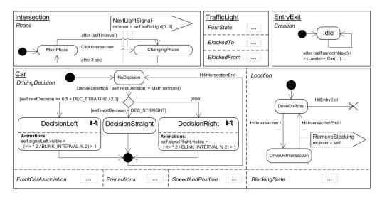
Figure 4: *AML* model: state machines and animation behavior (excerpt)
