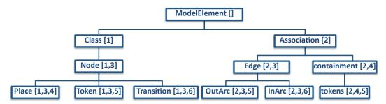
Figure 7: The Type System of the Petri net Simulator (without built-in types)
