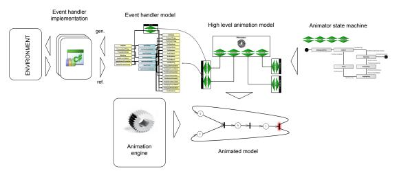
Figure 1: The Architecture of the VMTS Animation Framework
