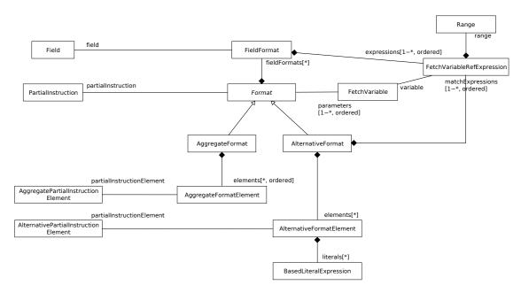
Figure 4: Extract of the HARMLESS metamodel: instruction binary format modeling
