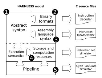
Figure 1: Processor views and simulator generation using HARMLESS
