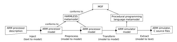
Figure 12: Simulator generation from HARMLESS models
