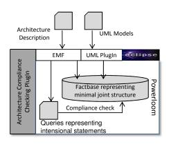
Figure 5: Structure of the prototypical tool.
