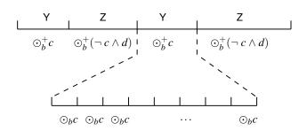
Figure 6: Execution of program  $\langle c \to Y, d \to Z \rangle \dagger b$  with guard approximation
