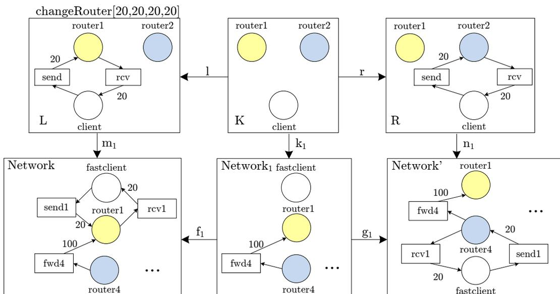
Figure 6: Application of rule  $changeRouter$  (injective matching)
