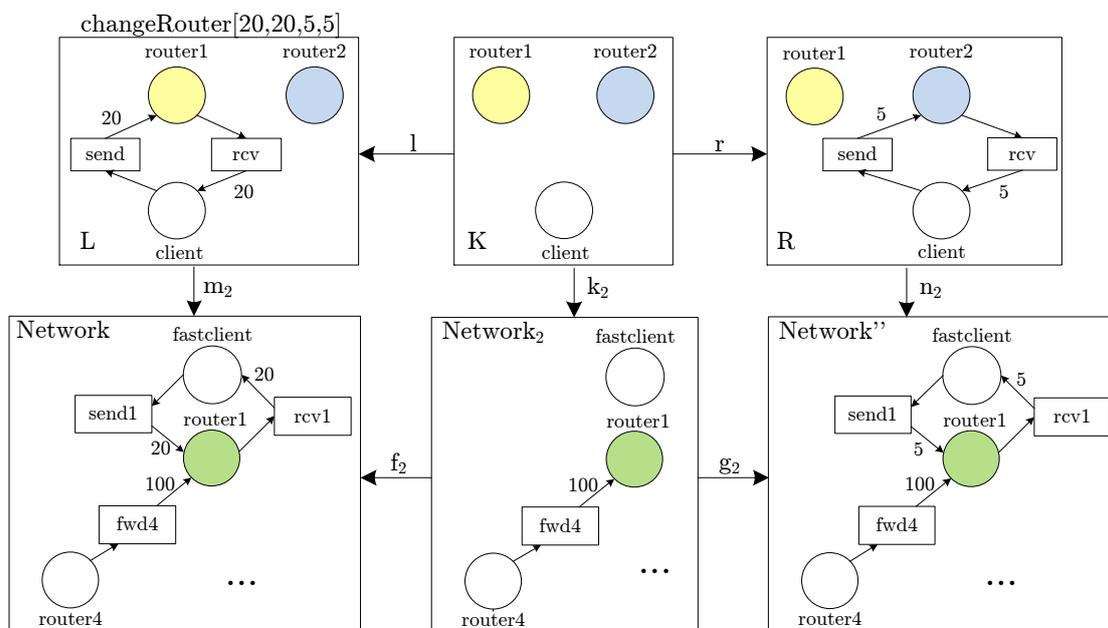
Figure 7: Application of rule *changeRouter* (non-injective matching)
