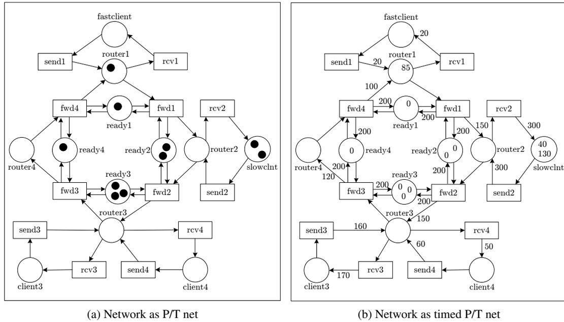
Figure 1: Network as P/T net and timed P/T net
