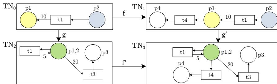
Figure 4: Gluing and restriction of timed P/T nets
