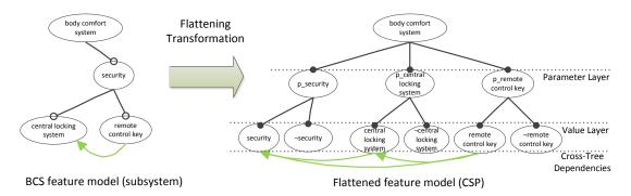
Figure 4: Parameter and Value Layer for a BCS-Subset
