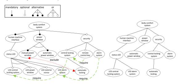
Figure 1: A feature model and a valid product configuration in concrete syntax.
