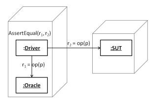
Figure 1: Oracle implementation schematic diagram
