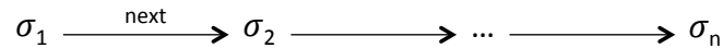
Figure 1: Execution of a model by a MoC. \sigma_i is an observation of the state of the model.
