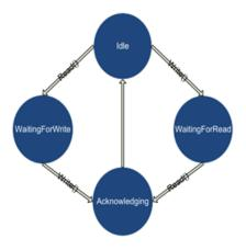
Figure 3: Definition of Synchronous Communication with FSM
