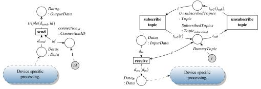
Figure 5: AHLI nets for asynchronous devices
