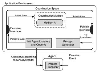
Figure 2: Conceptual model of Coordination Spaces [VSL+10].
