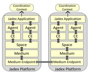
Figure 4: Realization of Peer-to-Peer Coordination Spaces in Jadex
