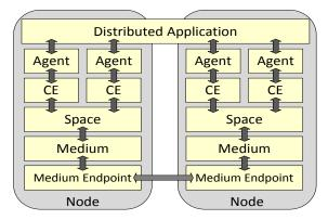
Figure 3: Peer-to-Peer Coordination Spaces architecture
