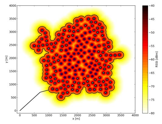
Figure 1: A typical run of the algorithm for a typical node placement is depicted. Shown are the nodes as dots where their color denotes if they have been visited or not. Cyan nodes were in communication range of the robot and blue nodes were not. Additionally, the maximum RSSI value from all nodes is shown for every point as the underlying color plot. The black line is the path the robot took in this run. In the shown simulation the measurements of the robot were noise-free.
