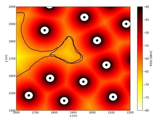
Figure 2: A situation is shown where the robot got stuck in a narrow cavity between several nodes forming some kind of cavity inside of the network. As can be seen, the robot does one additional turn before it can escape this situation. This is a fully random process since it is mainly due to the noise in RSSI measurements. The black line is the path the robot took, the nodes are shown as black dots and the maximal RSSI value from all nodes is shown for every point as the underlying color plot.
