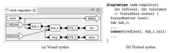
Figure 2: A regulator model for a tank with two input parameters (refLevel and tolerance) and one output parameter (status). White rounded rectangles represent blocks. Sub means subtraction, Neg negation, and GTZ means greater than zero and returns a boolean value. A valve takes a boolean value, indicating if it should be open or not. The data flow is from left to right.
