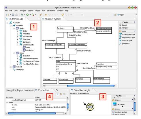
Figure 4: VL Design of the Automata VL with the TIGER Designer
