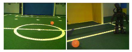
Figure 4: Two images taken and processed by a humanoid soccer robot on a standard RoboCup field [LR07]. The colored dots and lines indicate perceived parts of goals and field lines; the recognized ball is bordered by an orange circle.
