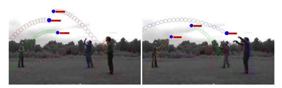
Figure 10: Camera view of the tracking scenario and overlaid detection results (red circles) and predicted ball trajectories (coloured circles).
