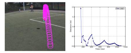
Figure 9: Predicting the trajectory of a flying ball from a moving camera-inertial system. As an initial study, the ball, the lines, and the goal corners have been manually extracted from the images. From this data, the trajectory of the ball is predicted (left). The right plot shows the error of the predicted touchdown point varying over time. It shows that, even though the camera is moving, the prediction is roughly precise enough for interception.
