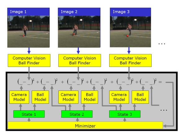
Figure 5: Information flow in a ball tracker based on the conventional data-driven paradigm (see text). The ball finder is not part of the optimization loop (gray box).
