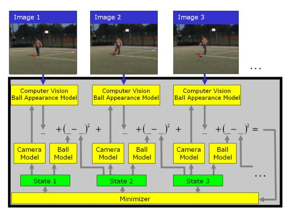
Figure 6: Information flow in a ball tracker based on the global likelihood optimization paradigm (see text). Here, computer vision, i.e. the ball appearance model, is part of the optimization loop (gray box).
