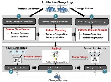
Figure 2. Overview of Proposed Solution – Change Mining (PatEvol Development) and Change Execution (PatEvol Application).
