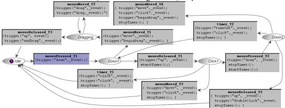
Figure 3 – ICO mouse transducer model
