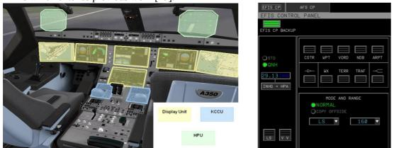
Figure 1 - Example of an aircraft cockpit and screen shot (left) of a WIMP aircraft application (right)
