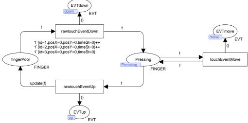
Figure 8 - CPN translated low level event transducer model
