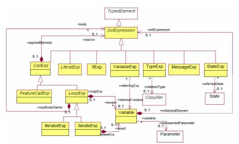
Figure 7. The basic structure of expressions in the OCL metamodel
