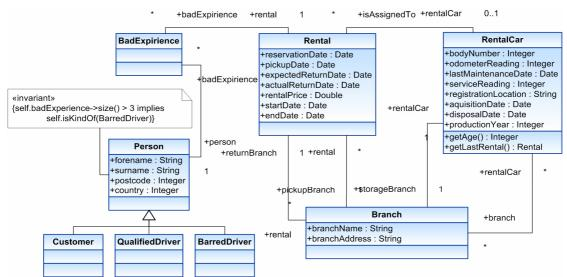
Figure 1. OCL invariant and its corresponding UML class Person in the UML class diagram
