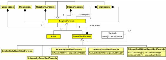
Figure 5. The concept of a logical formula in R2ML
