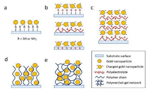
Figure 1. Various surfaces along with nanoparticles used in immobilization.
