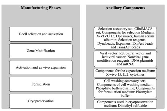
Figure 4. Manufacturing phases of CAR T cell manufacturing and various ancillary components required in those phases.
