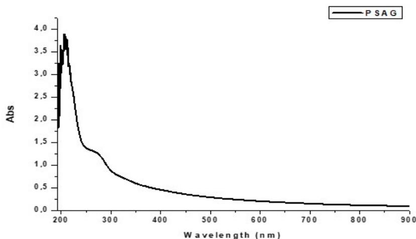
**Figure 2.** Uv-vis absorption spectra of PSAG (polysaccharides extracted from *Astragalus gyzensis* Bunge. seeds).
