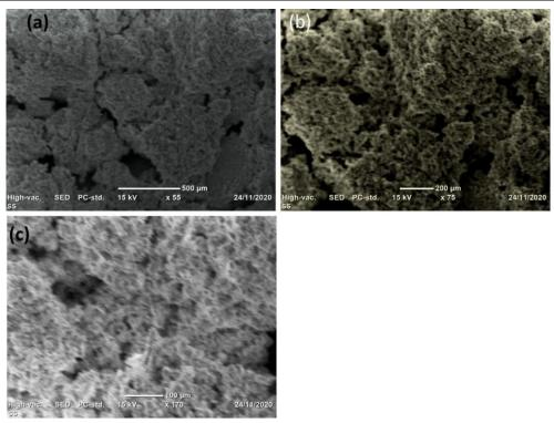
**Figure 3**: The SEM images of silica micro particles in different resolution of (a) 500 μm, (b) 200 μm, and (c) 100 μm.
