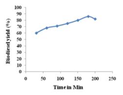
Fig.8. Effect of Reaction time
