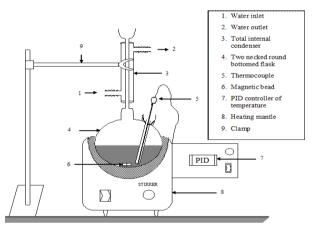
Fig.2. Schematic Diagram of the Experimental Setup
