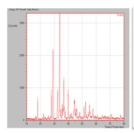
Figure.3: XRD of Manganese Carbonate.
