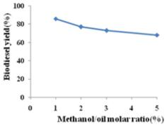
Fig.5. Effect of methanol/oil molar ratio
