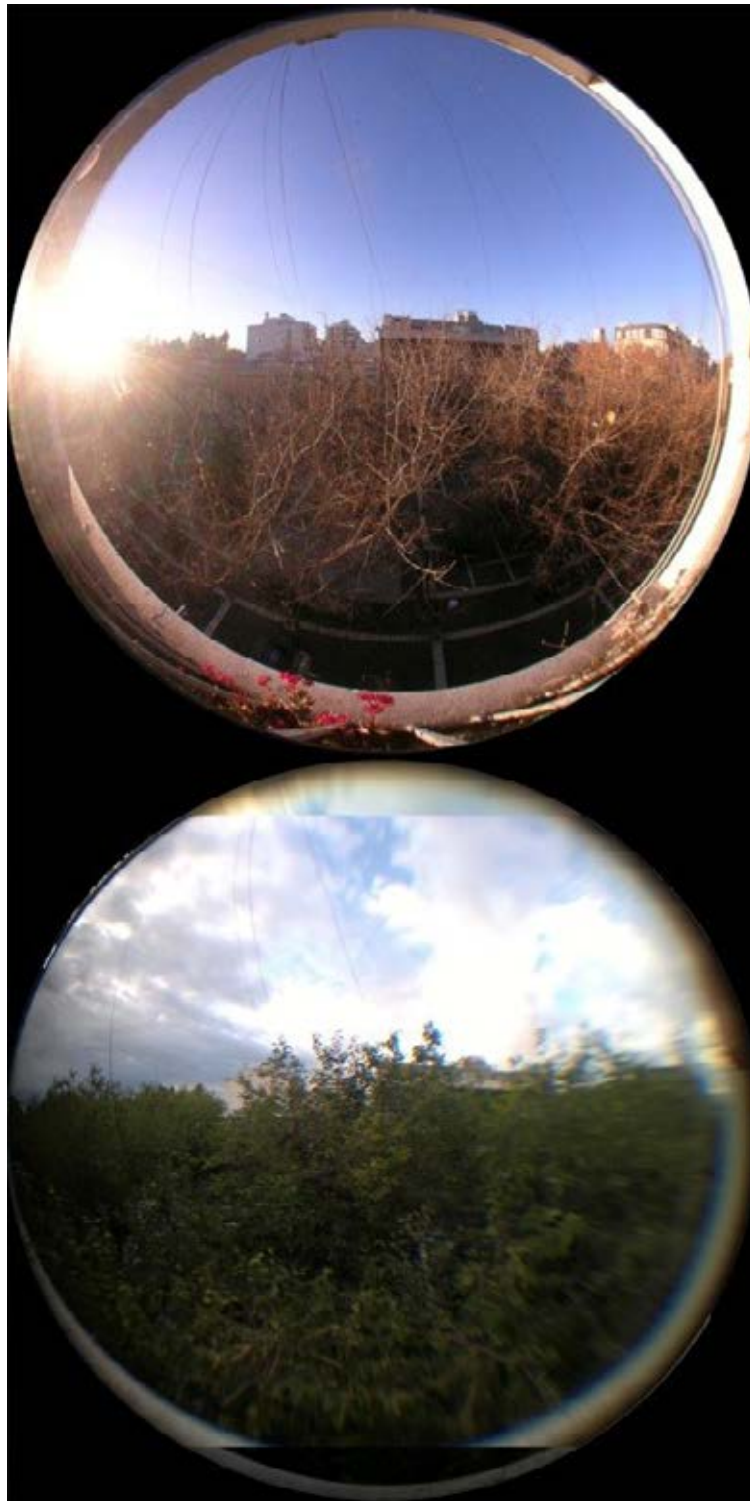
Figure 5. Hemispherical photographs of the environment, taken from the sensor location. Case 1. Facade zone with partial insolation. Third floor.
