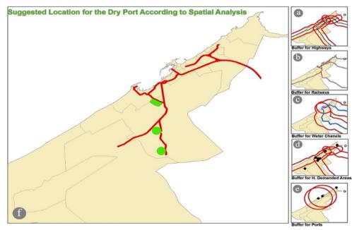
Figure 8. The suggested location for the dry port according to spatial analysis.
