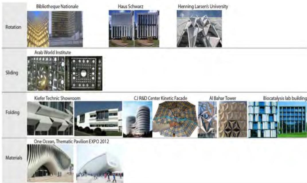
Figure 5. Examples of different kinetic facades' motion and mechanism (source: El-Dbaa, 2016)
