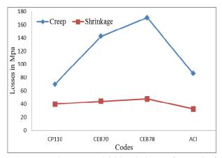
Fig. 4. Losses due to creep and shrinkage in the case of post-tension for different codes.
