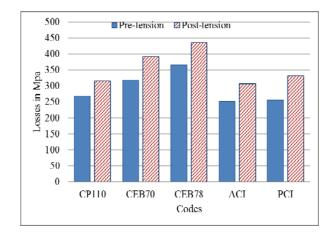
Fig. 1. Comparison of Total Losses between Pre-tension and Post-tension.
