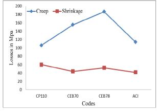
Fig. 3. Losses due to creep and shrinkage in the case of pre-tension for different codes.
