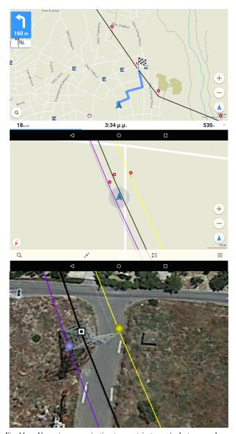
Fig. 11. Upper image: navigating to a certain tower (only tower and axes shown). Middle image: reaching the tower (turning on all placemarks). (Screenshots from Mapswithme/Maps.ME version 6.5.2, Map data from OpenStreetMap). Lower image: View of the tower in Google Earth Pro (Screesnshot for Google Earth Pro, Map data: Google).
