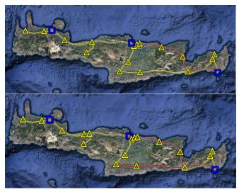
Fig. 2. The power system of Crete in 2016. Up: current scheme, Down: near future scheme. Squares denote power plants and triangles denote step down substations. Red line denotes a double circuit and yellow line denotes a single circuit. (Screenshots from Google Earth Pro, Map data: Google, Image LandSat, Data SIO, NOAA, U.S. Navy, NGA, GEBCO)
