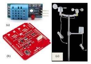
Fig. 4. Weather shield, DHT11, and wind-rain sensor.
