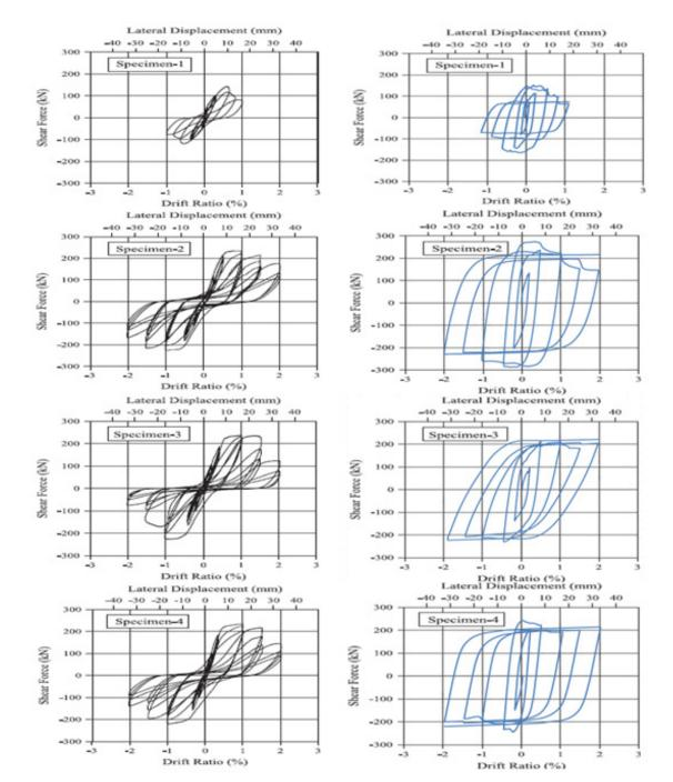
Fig. 7. Force-drift hysteresis curve under cyclic load, Group C - Specimens 1-4 a) experimental b) numerical
