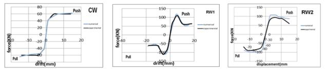
Fig. 5. Push comparison of hysteresis curves of experimental results and numerical analysis for Group B specimens.
