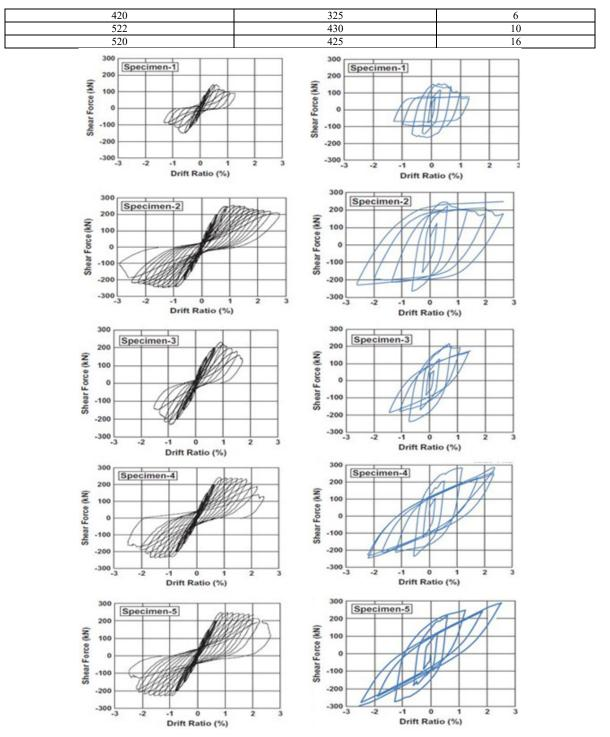
Fig. 1. Force-drift hysteresis curve under cyclic load, Group A, Specimens 1-5 a) experimental b) numerical
