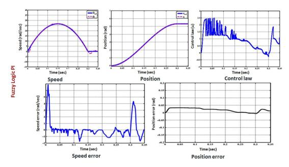
Fig. 5. Simulation results for fuzzy logic PI controller
