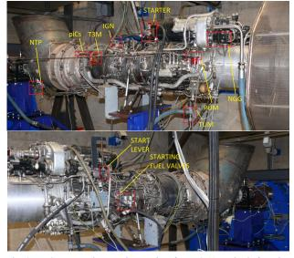
Fig. 6. Sensors and Measuring Devices for TV2-117 turboshaft engine
