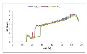
Fig. 12. Fuel flow variation with engine speed
