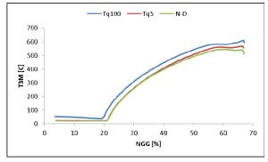
Fig. 9. Inlet Turbine Temperature variation with engine speed
