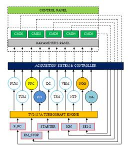
Fig. 3. TV2-117A Instrumentations and acquisition system
