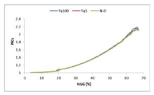
Fig. 10. Static overall pressure ratio variation with engine speed
