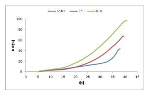
Fig. 15. Free turbine speed variation with starting time
