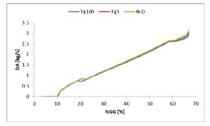
Fig. 11. Air flow variation with engine speed
