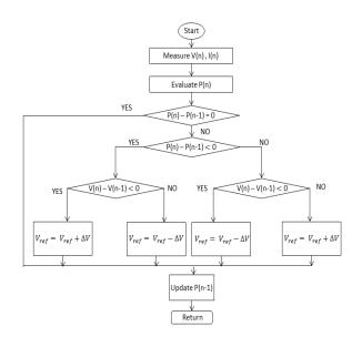
Fig. 8. The flow diagram of the P&O method.
