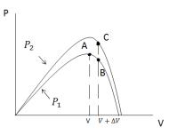
Fig. 9. Separation diagram of MPP for P&O.
