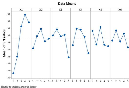
Fig. 1. Main effects plot for S/N ratios for Pb extraction (dashed line indicates mean value)
