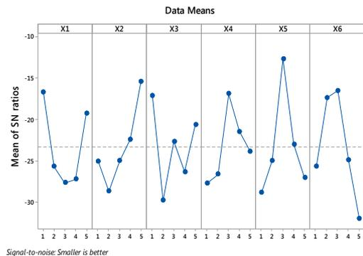
Fig. 2. Main effects plot for S/N ratios for emulsion breaking (dashed line indicates mean value)
