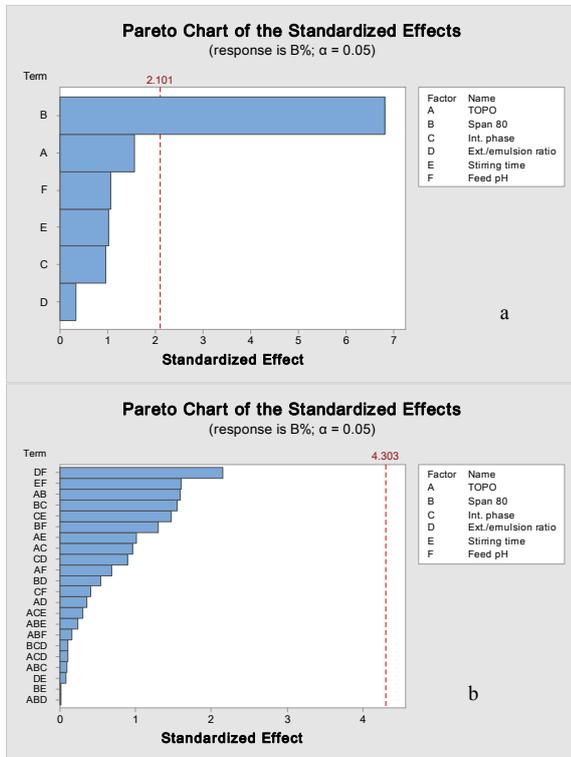
Fig. 4. Pareto chart of a. independent parameters, b. interaction effects of ELM parameters on emulsion breaking.
