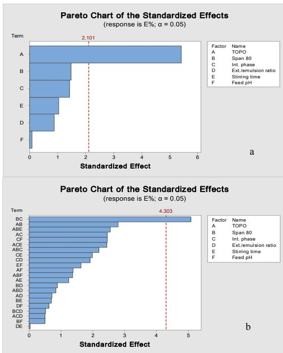
Fig. 3. Pareto chart of a. independent parameters, b. interaction effects of ELM parameters on extraction of lead.
