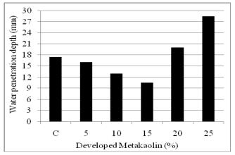
Fig. 2. Water penetration of ordinary and metakaolin concrete
