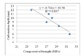
Fig. 7. Relationship of compressive strength and carbonation depth of metakaolin concrete
