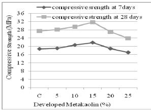
Fig. 1. Compressive strength of plain (C) and Metakaolin concrete
