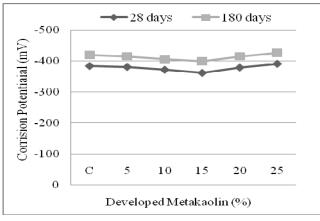
Fig. 3. Corrosion potential of ordinary and metakaolin concrete
