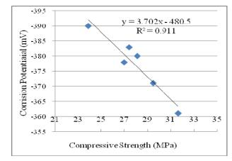
Fig. 6. Relationship of compressive strength and corrosion of metakaolin concrete
