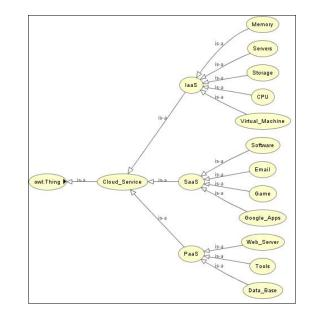
Fig. 5. Ontology Model of the Cloud Services based on OWLViz Chart
