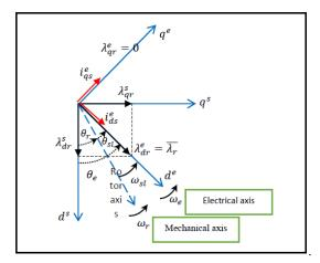
Fig. 5. The rotor flux oriented vector control diagram
