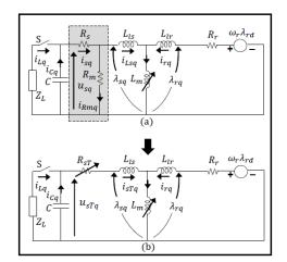
Fig. 2. The equivalent circuit of the SEIG
