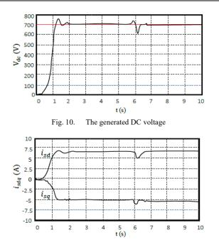
Fig. 11. Changes in the d and q components of the stator current
