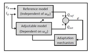
Fig. 6. The main structure of the model reference adaptive system
