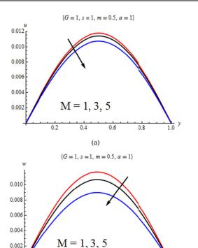
(b) Fig. 3. (a) Primary velocity profile and (b) Secondary velocity profile for different  $\mathbf{M}$
