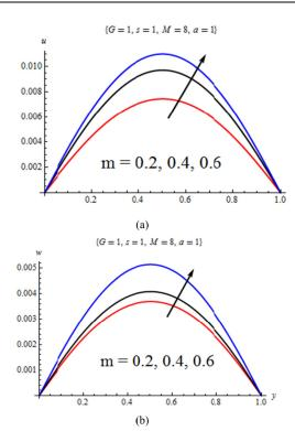
Fig. 1. (a) Primary velocity profile and (b) Secondary velocity profile, for different  $\boldsymbol{m}$
