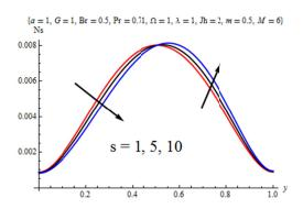
Fig. 9. Entropy generation profile for different s
